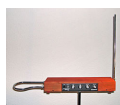
Fig. 14: A Moog Etherwave, assembled from a theremin kit: the loop antenna on the left controls the volume while the upright antenna controls the pitch.
